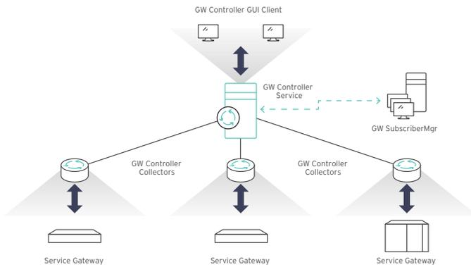
**Interface Layer:** Provides multiple levels of access/operation, and open interfaces for integration with external systems.
